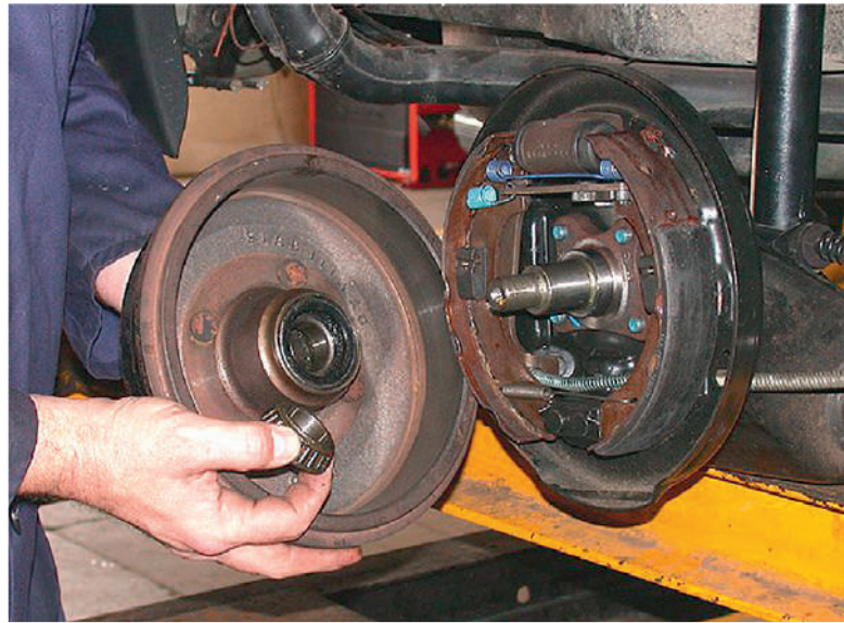
Figure 5.102 Rear hub (dead axle) with taper bearing
